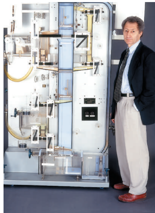
A. W. Phillips built this model in the early 1950s to illustrate Keynesian theory.
